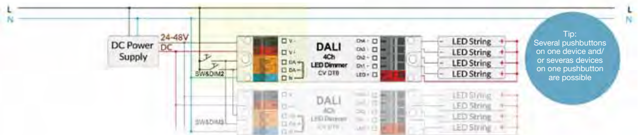
Connection example: LED dimmer control via push button (SW&DIM2)
