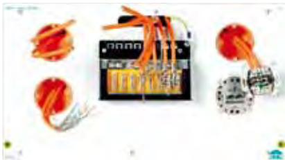
Patch Panel Board
