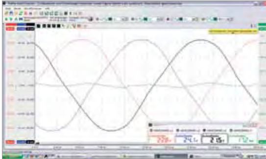
Unsymmetrical load, L1 low-resistance, neutral conductor closed
