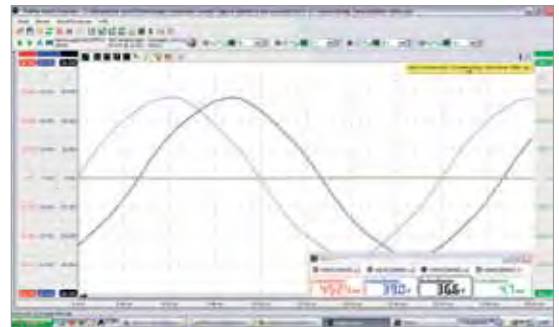
Unsymmetrical load, L1 low-resistance, neutral conductor open
