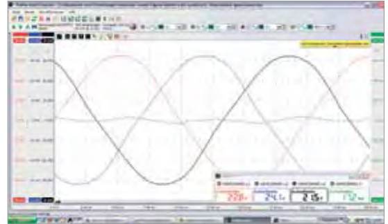
Symmetrical load, neutral conductor closed
