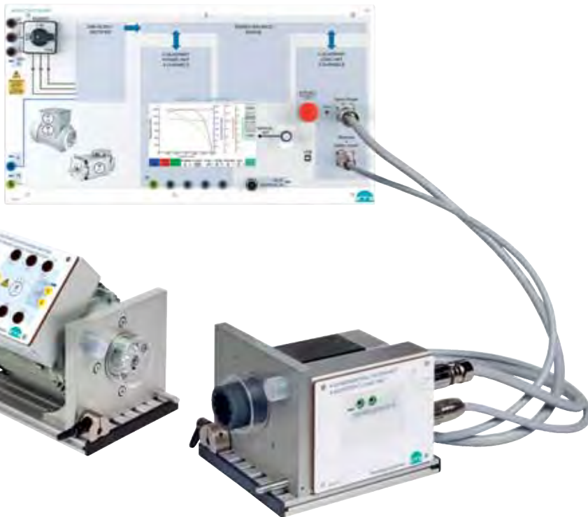
Modern power electronics applied in the ETS motor test bench.
